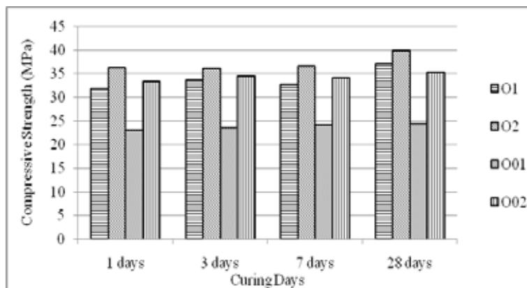
Figure 6. Compressive strength results of oven curing geopolymer concrete
