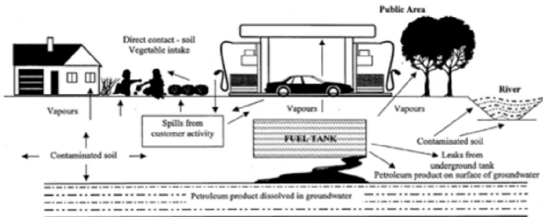
**Figure 2.** Fuel Leaks and Spills possibly Contaminate Soil dan Grounwater
