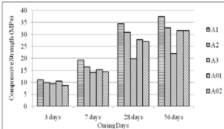
Figure 5. Compressive strength results of ambient curing geopolymer concrete
