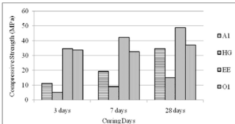
Figure 7. Comparison between each curing method
