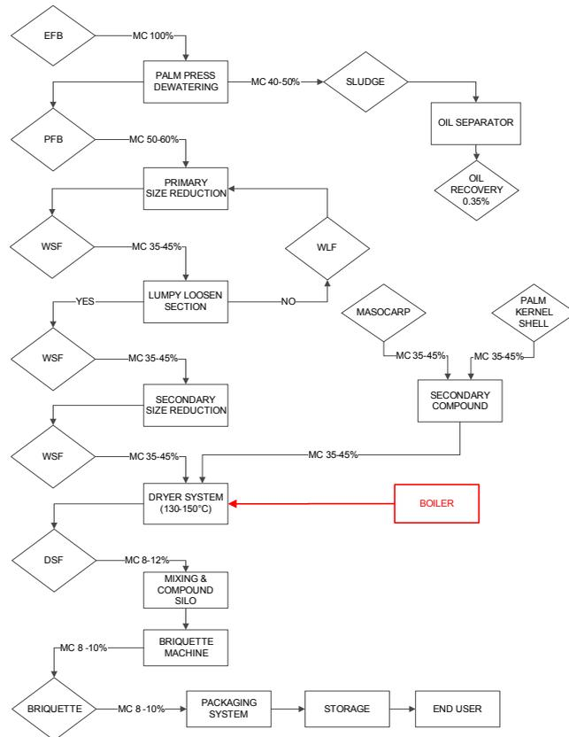
**Figure 1.** Process flow diagram of the solid bio-fuel briquettes production
