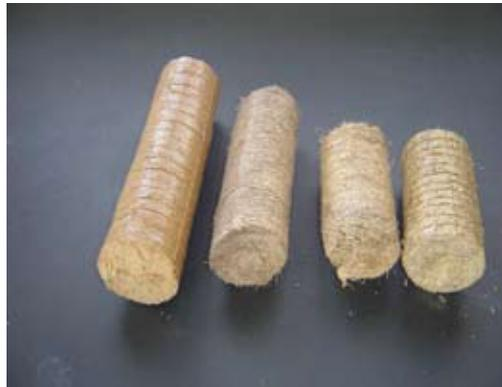
**Figure 3.** Palm-based solid bio-fuel briquettes
